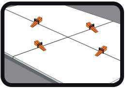
2. Slide the FORPAC® Wedge through the opening of the each Spacer Clip to ensure your tiles are leveled. Tighten the wedge either with hand or rubber mallet.
