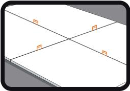
1. After placing the tile on the floor proceed placing the FORPAC® Spacer Clip two inches away from each corner of the tile.
